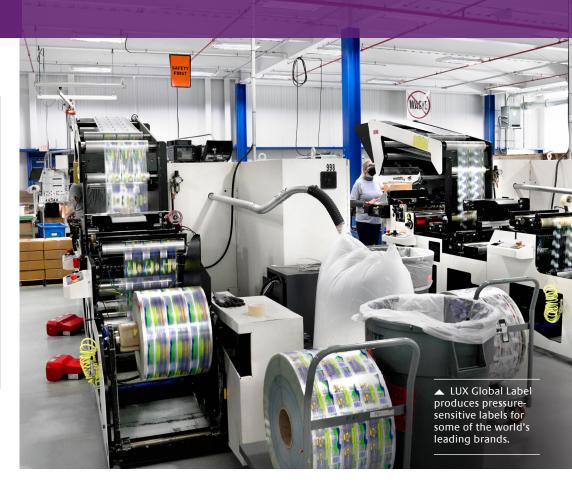
The installation of the HS-Web hardware was done in one day on LUX Global Label's rewinder. The system's eight-camera setup allows for capture of up to 16 lanes across and 25,000 signatures per minute. It works in line with the existing manufacturing process—capturing at standard rewinder speeds.
